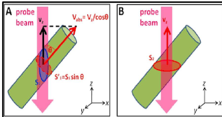
**Figure 9: Light of laser Doppler imaging inside target and principle of produce Doppler shift.**
