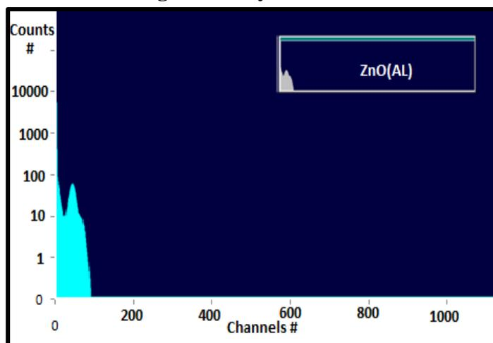
**Fig. b.** Pulse height spectra of 3mm ZnO(Al) ceramics for 59.54-keV gamma-ray from  $^{241}\text{Am}$ .
