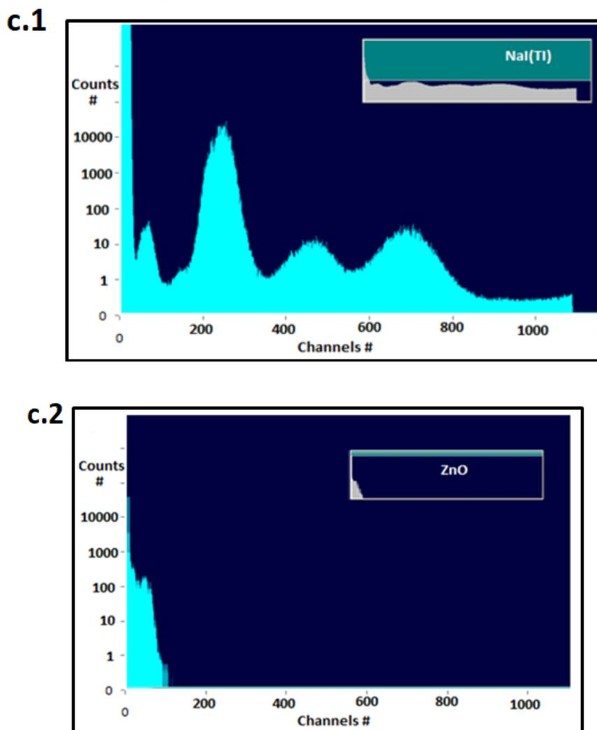
**Fig. c.** Pulse height spectra of (c.1) NaI(Tl) and (c.2) undoped 3mm ZnO ceramics for gamma-ray from  $^{152}\text{Eu}$ .
