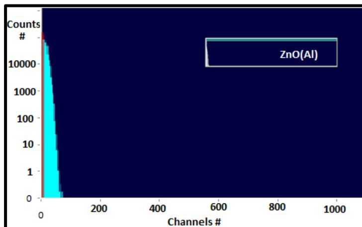
Fig. d. Pulse height spectra of 3mm ZnO(Al) ceramics for gamma-ray from  $^{152}\text{Eu}$ .
