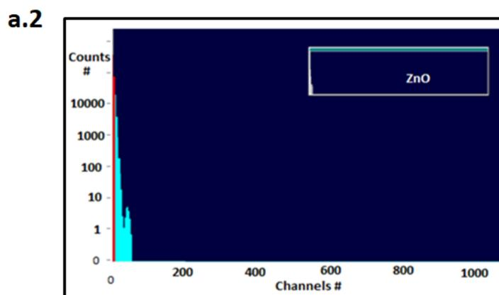
**Fig. a.** Pulse height spectra of (a.1) NaI(Tl) and (a.2) undoped 3mm ZnO ceramics for 59.54-keV gamma-ray from  $^{241}\text{Am}$ .
