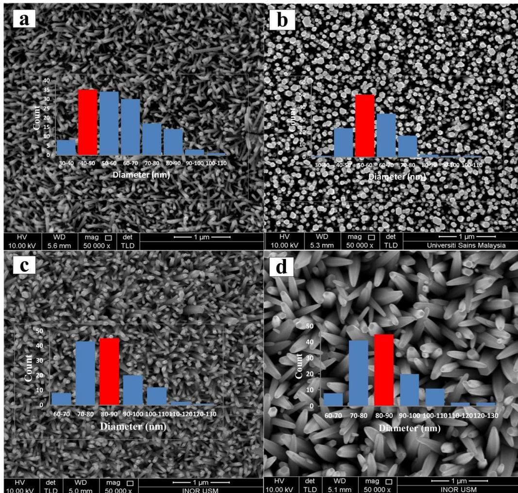
Fig. 2. FESEM images of the ZnO nanorod arrays with different precursor concentrations: (a) 10m M, (b) 25m M, (c) 50m M, and 75mM.
