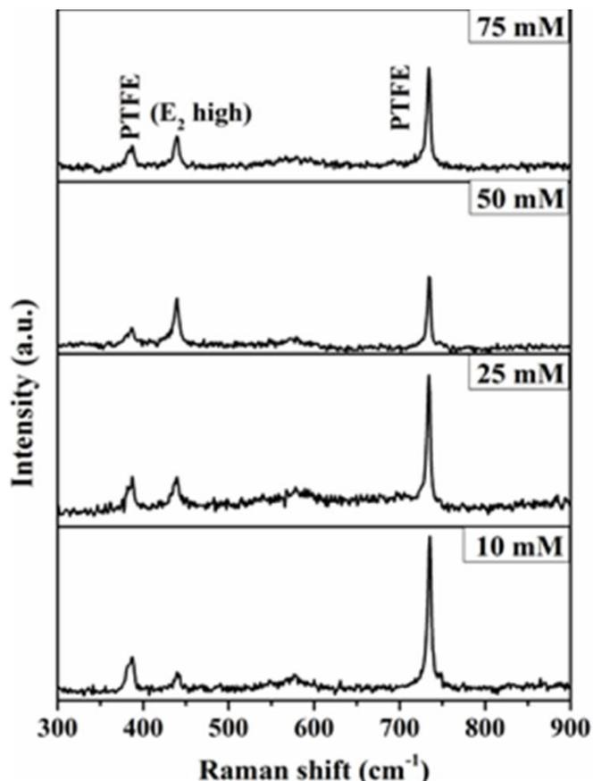
Fig 3. reveal the Raman spectra for ZnO nanorod array that were prepared by using precursors of different concentration on PTFE
