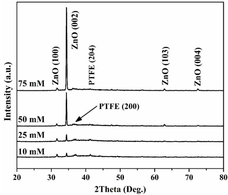
Fig. 1. XRD patterns of the ZnO nanorods with various precursor concentrations: (a) 10 mM, (b) 25 mM, (c) 50 mM, and (d) 75 mM.
