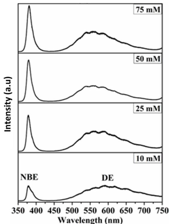
Figure 4: Photoluminescence (PL) of ZnO nanorod array grown from a precursor of different concentration on PTFE substrate.
