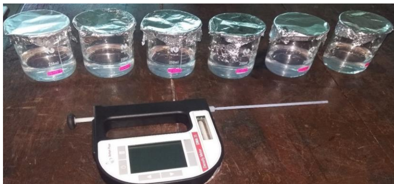
Figure 3: Electronic Density Meter (DMA35) for samples density measurements.
