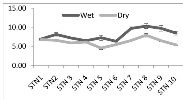
**Figure 4: Biochemical oxygen demand (mg/L)**
