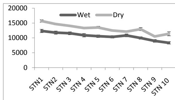
**Figure 2: Total dissolved solids (mg/L)**
